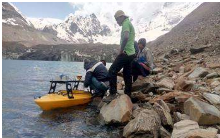
Photo -1 : Bathymetry survey on Gepang Gath Lake using RCV boat fitted with echo-sounder and GPS
