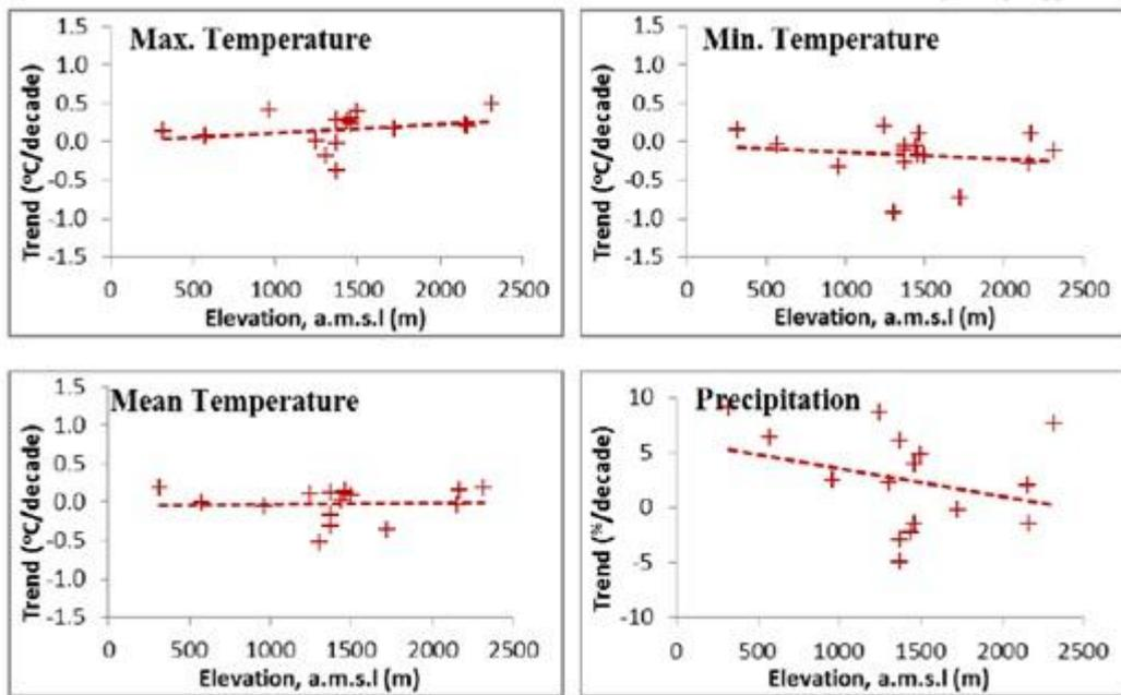
**Figure 5-6: Distribution of trends of precipitation, mean, maximum and minimum temperature with elevation.**
